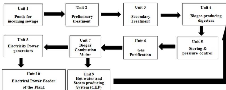
Fig 2. Schematic view of the units under control
